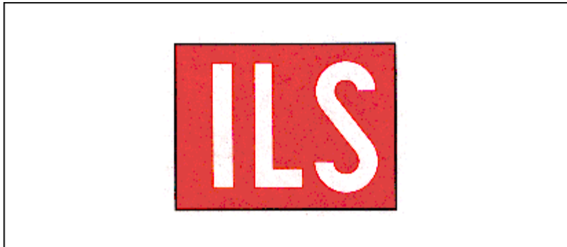
FIG 2-3-29 Sign Prohibiting Aircraft Entry into an Area
